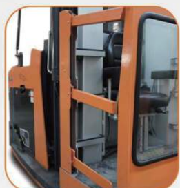
The cabin is equipped with two electronically locked grille doors for safety and stability to prevent accidents.
