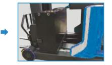
■In order to replace the battery its tray should be reached forwards. The mechanism for battery's tray release is located near with operator's foot.
